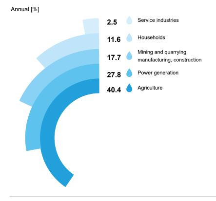
In the case of Poland, power generation is the largest industrial demand for water, accounting for approximately 25% of the country's annual water consumption. Water is primarily used in coal-fired power plants to cool the power units. In order to manage the available resources rationally, it is worth considering in which areas of economic activity, apart from the previously mentioned power generation, the greatest consumption occurs.
